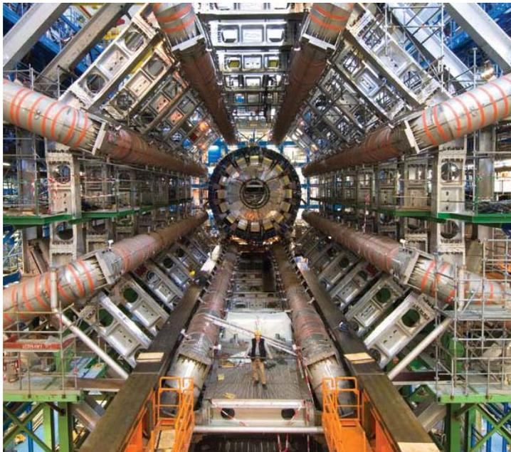
***The ATLAS detector in the first stages of construction. One can see the huge octagonal magnet enveloping it. The magnet's job is to bend muons (heavy electrons) that leave the detector, in order to measure their energy. Image: CERN***
